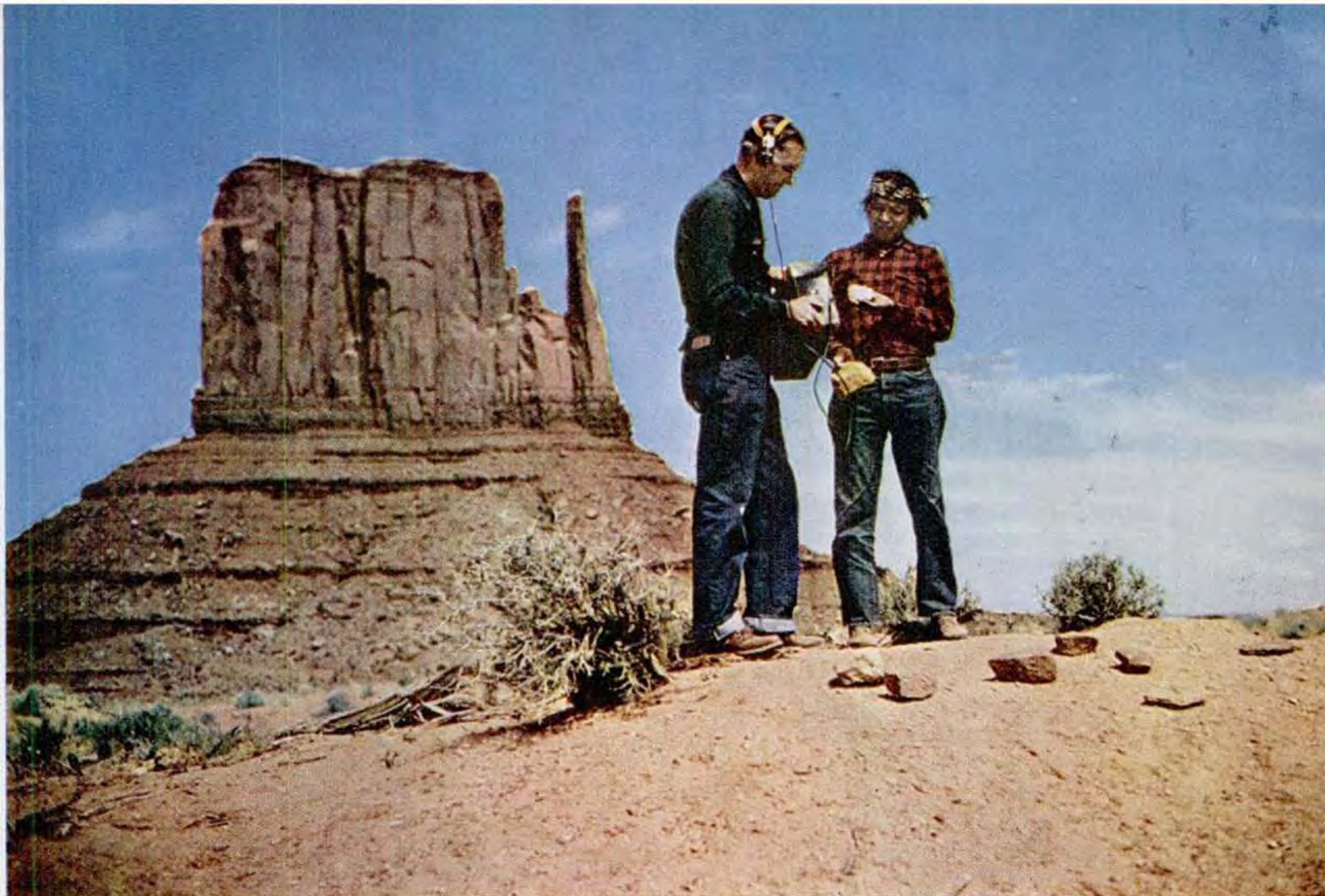
Trader Goulding shows Navajo prospector how a Geiger counter reveals radioactivity in piece of uranium ore Photos by Thomas E. Stimson, Jr.
